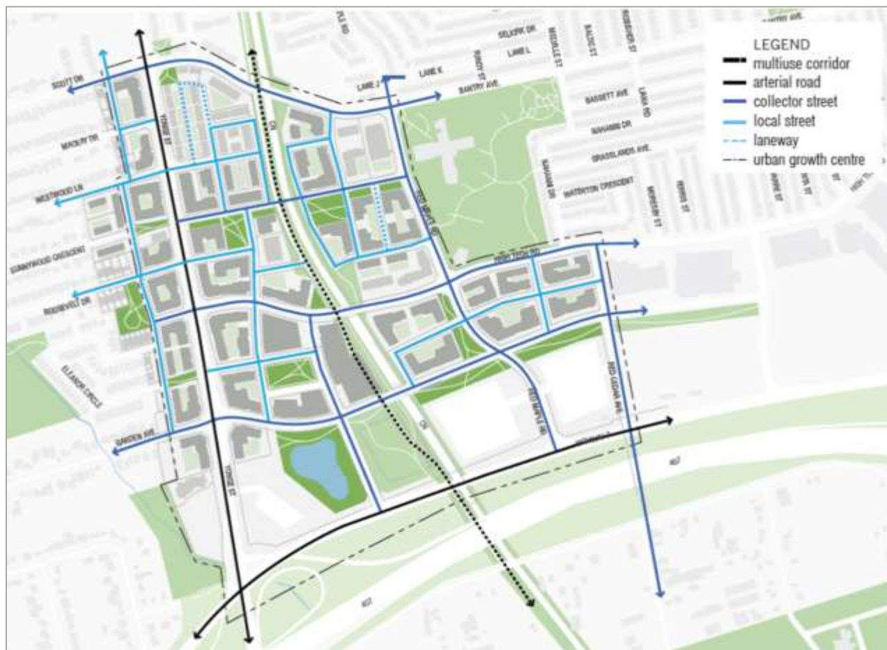
Figure 2-1: Richmond Hill Centre Recommended Road Network
