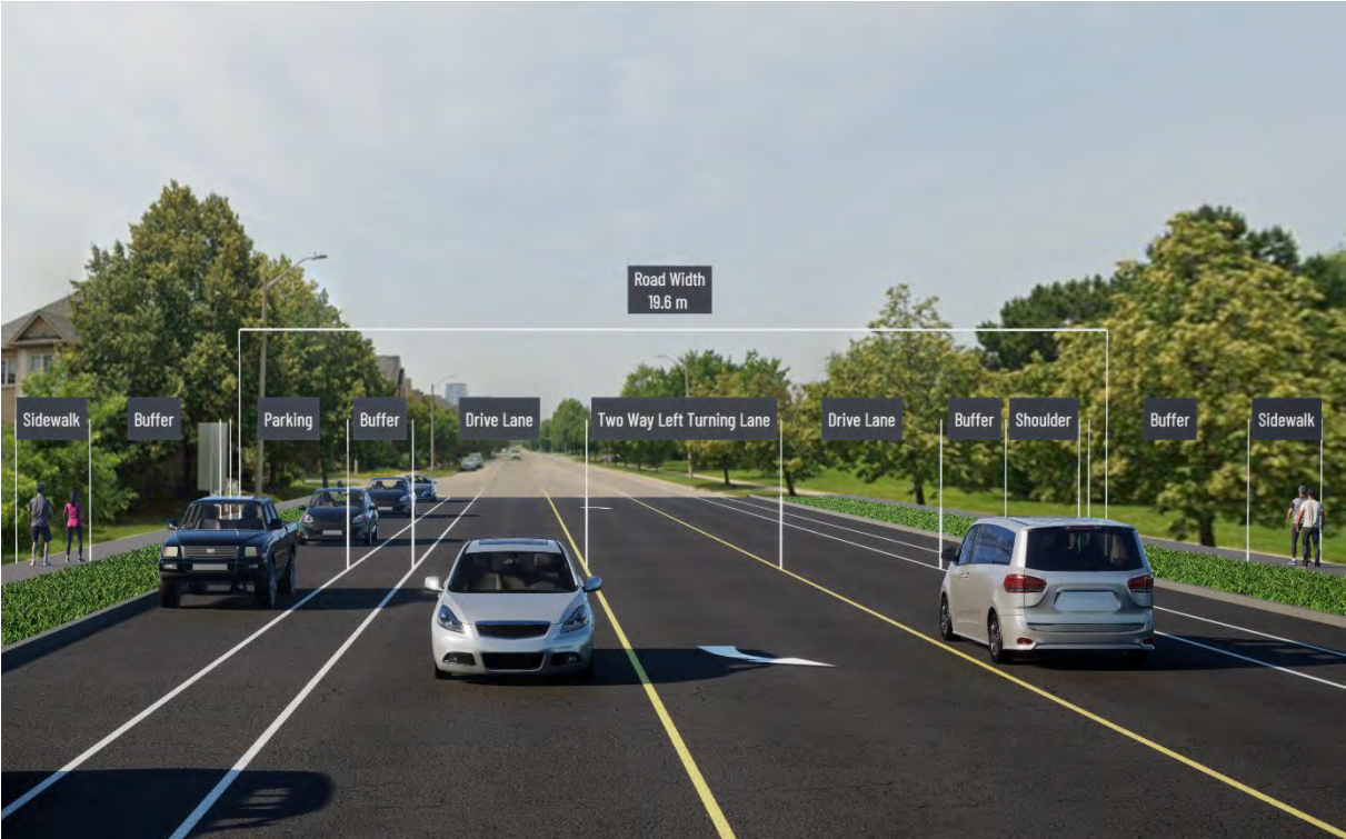
Figure 3-6: Existing Conditions on Bantry Avenue between Maple Road and Bayview Avenue – (Looking west)
