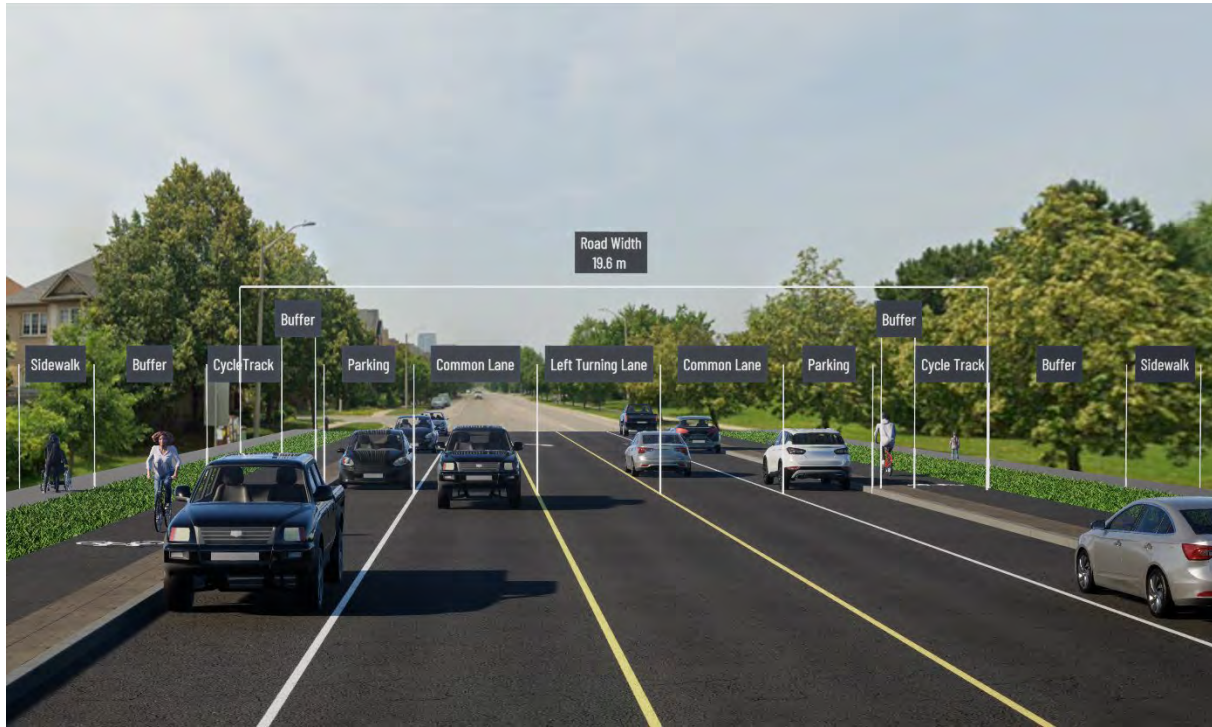
Figure 3-7: Corridor Option B1 – Cycle tracks on Bantry Avenue between Maple Road and Bayview Avenue – (Looking west)
