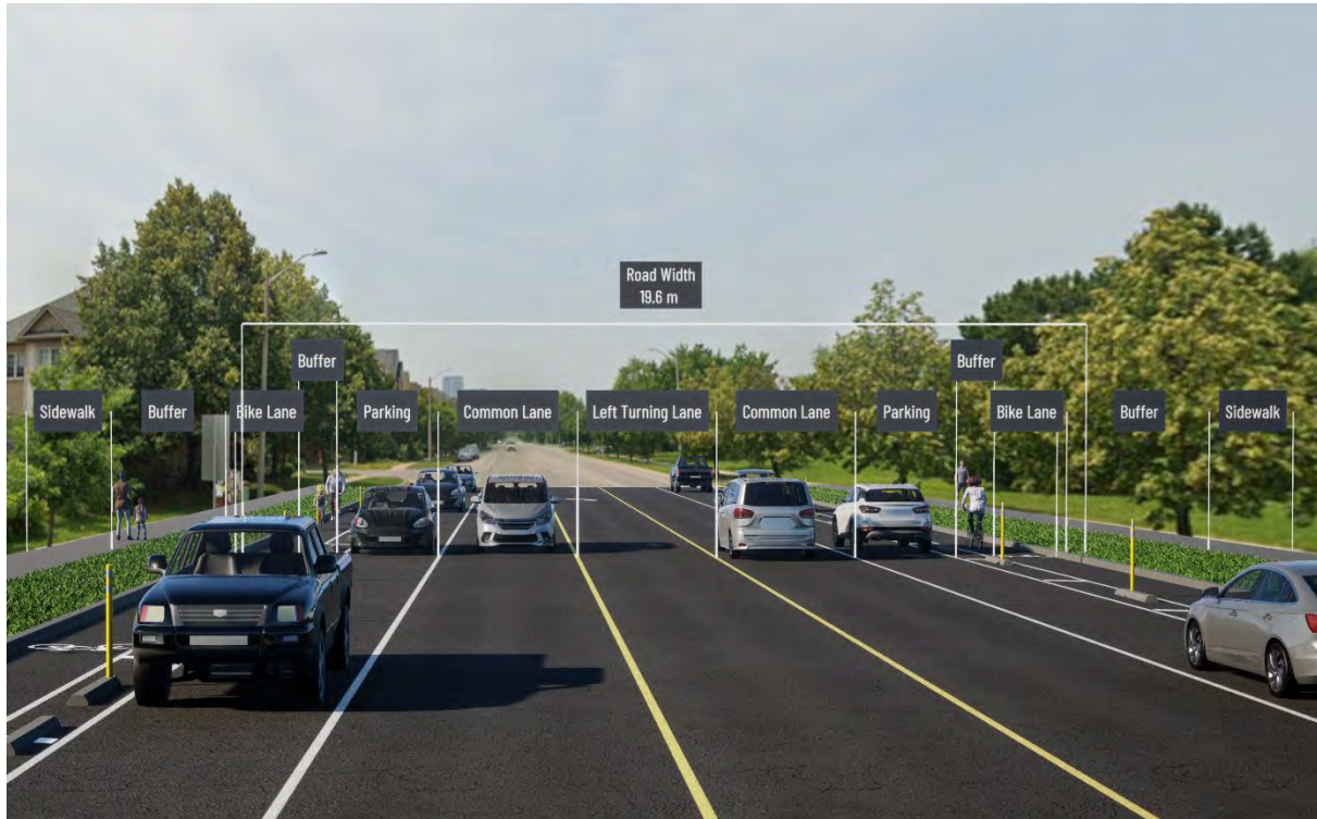
Figure 3-9: Corridor Option B3 – Protected bike lanes on Bantry Avenue between Maple Road and Bayview Avenue – (Looking west)
