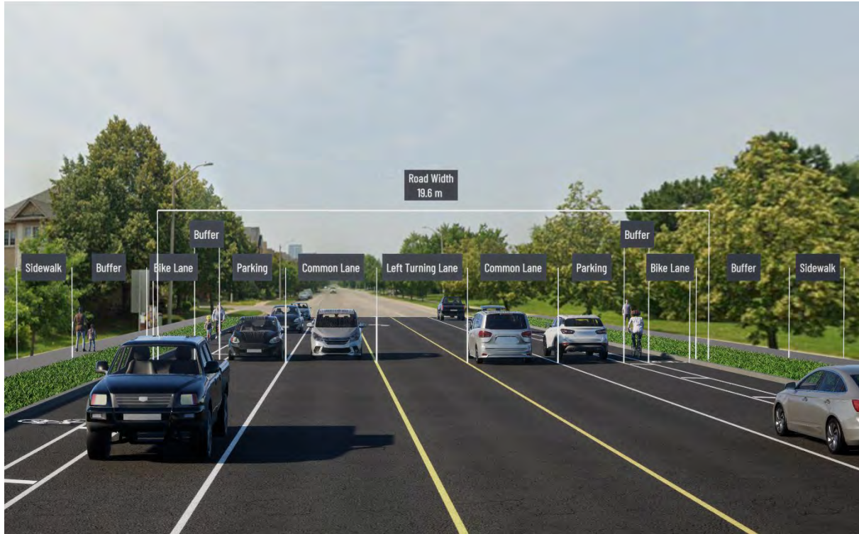
Figure 3-8: Corridor Option B2 – Buffered bike lanes on Bantry Avenue between Maple Road and Bayview Avenue – (Looking west)
