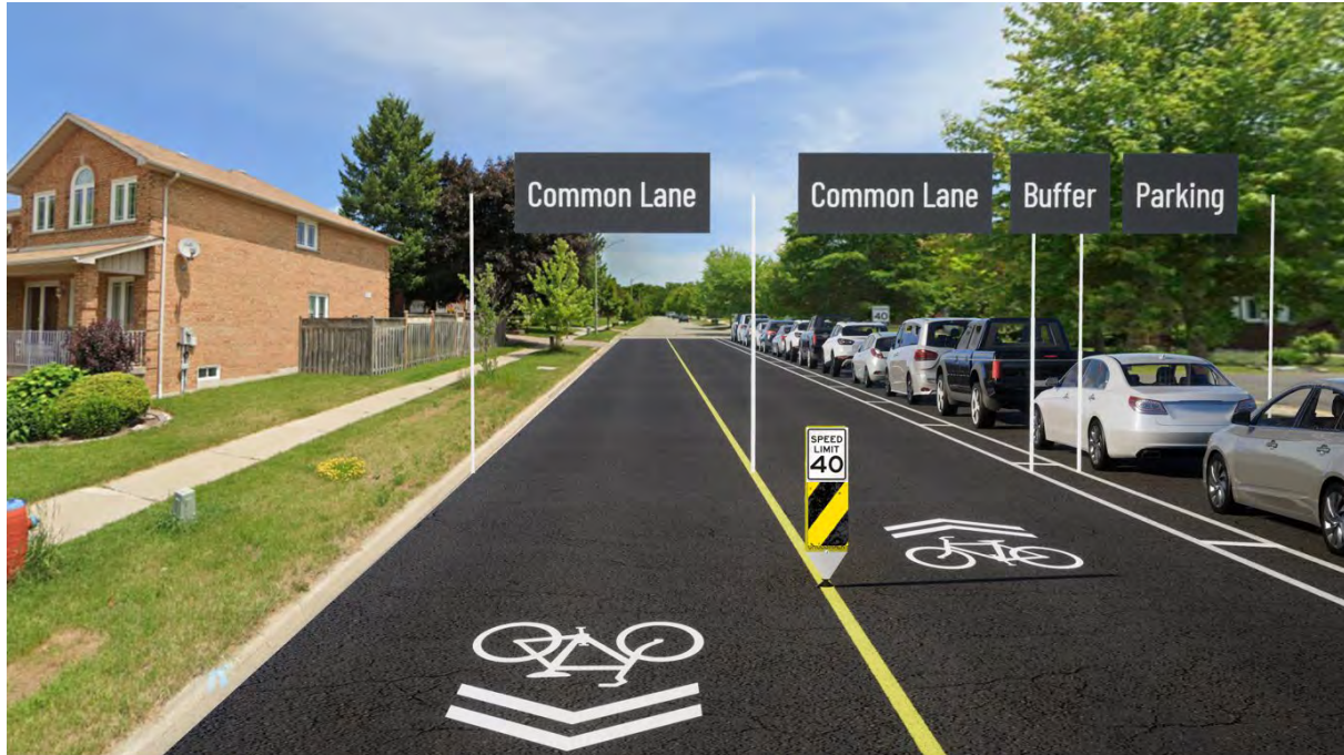
Figure 3-4: Corridor Option A2 – Shared Lanes on Briggs Avenue between Bayview Avenue and Edinburgh Drive – (Looking east)
