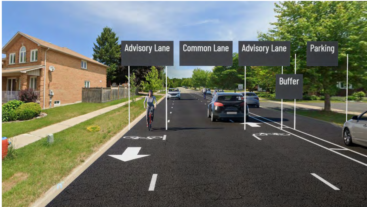
Figure 3-5: Corridor Option A3 – Advisory Bike Lanes on Briggs Avenue between Bayview Avenue and Edinburgh Drive – (Looking east)
