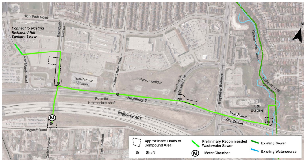
Figure 3-1 Regional Wastewater Servicing Plan (from Class EA)
